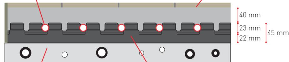
Lightweight screed. The surface must be flat and smooth, with max irregularity 0-4 mm.
