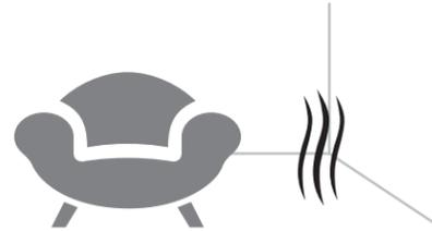
**Figure A** refers to convection systems, i.e. fan coils which generate forced air flows (convective motions) in the room; they cause the accumulation of masses of warmer air in the highest part of the room with consequent comfort problems for people, also because of noise levels and movement of particles.
