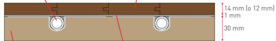
ECO DRY Floor Tech panel in wood fiber with pre-glued aluminum slats.
